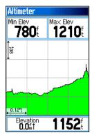
Altimeter Page displaying an Elevation over Distance Profile
